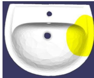
**Fig. 5:** Partially coated sink using intersecting points alpha shape
