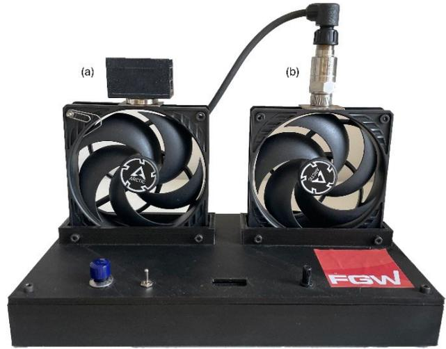
**Fig. 1:** A Test stand with two fans operating at the same frequency and two sensors: a MEMS sensor (a) and an IEPE sensor (b) mounted on the fan casing with a magnet. An intentional imbalance was introduced on the left side.
