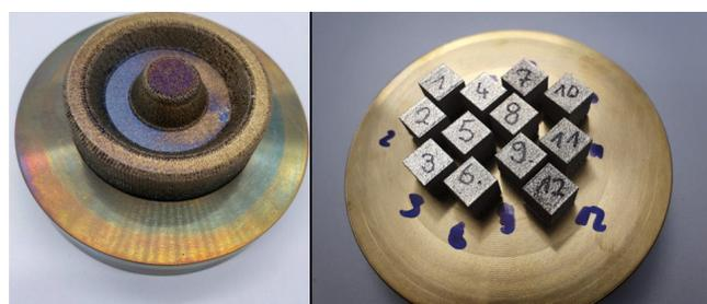
**Fig. 1:** a) Additively manufactured forging die without post-processing; b) Test print of cuboids for parameter determination.
