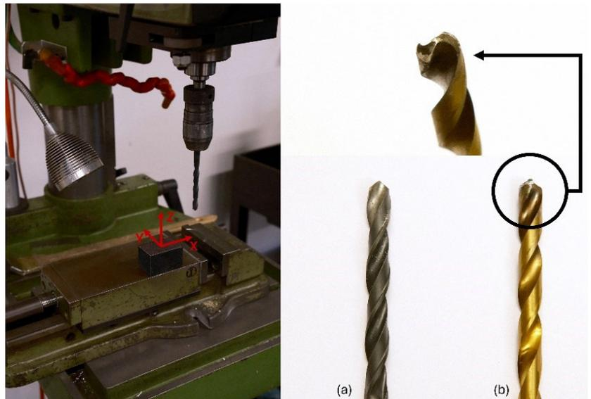
**Fig. 4:** Industrial drill setup with a smart sensor mounted on the clamping jaw using a neodymium magnet (left) and (a) a new drill and (b) a worn-out, defective drill with visible tip abrasions and cracks (right).
