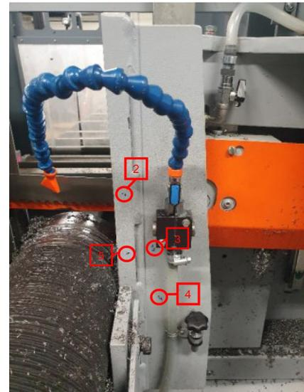
**Fig. 2:** Definition of several potential sensor positions at the bandsaw MEBA e-cut 400A.
