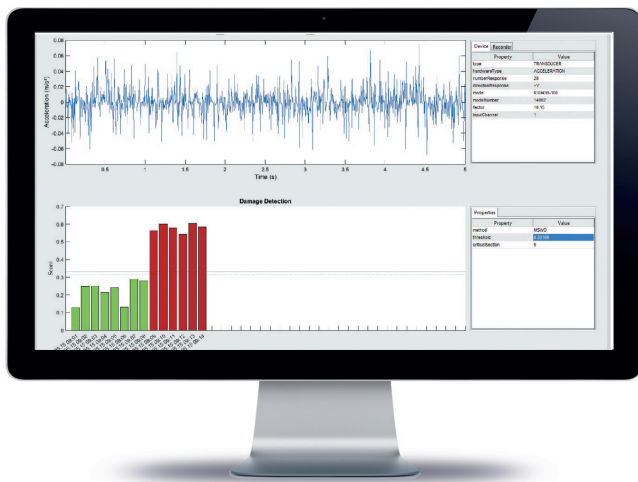
Fig. 1: Wavelmage Monitoring Software interface for online condition monitoring / quality control: green = no damage / red = damage
