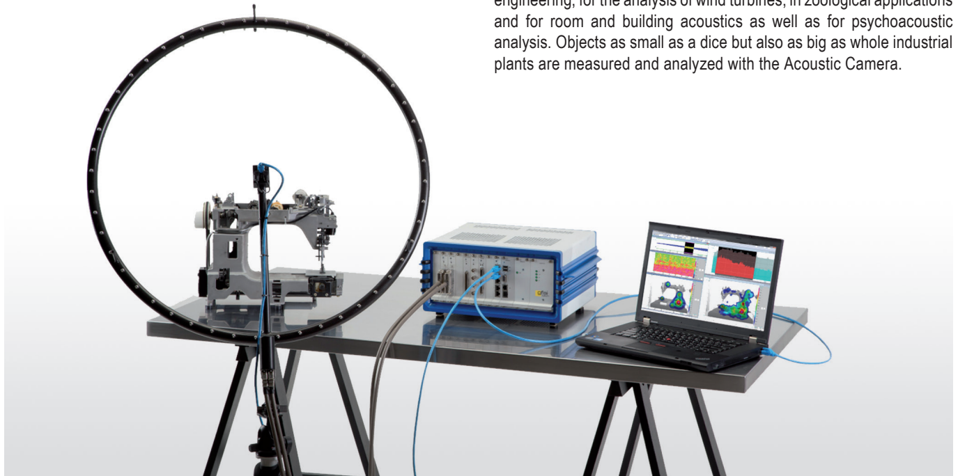
Typical Acoustic Camera system configuration: Microphone array, data recorder, laptop with NoiseImage (software for recording and post-processing)
