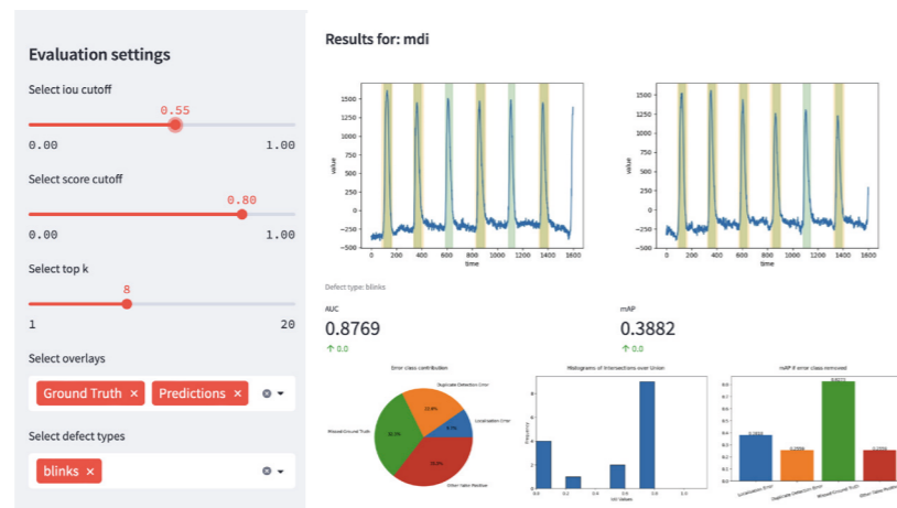
Fig. 3. (Left) The settings panel of TIADE (Right). We can see both the selected top-k and score-cutoff being applied to the time series viewer (red). Further, only the selected defect type (blinks) is considered.
