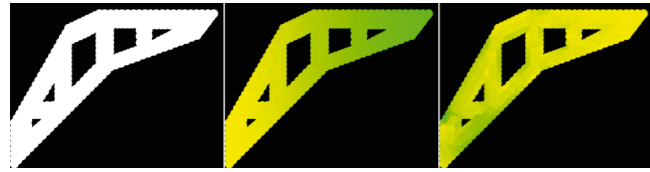
Fig. 6. Three images of the structural framework; the monochrome version, the displacement, and the von Mises stresses.
